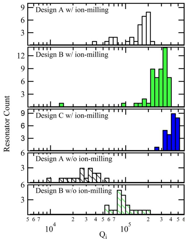
FIG. 4. Histograms of single-photon internal quality factors for designs A, B, and C resonators with ion-milling and designs A and B without ion-milling.  $Q_i$  improves steadily from design A to B to C. For both designs A and B resonators, when ion-milling is not performed,  $Q_i$  is roughly a factor of four lower.
