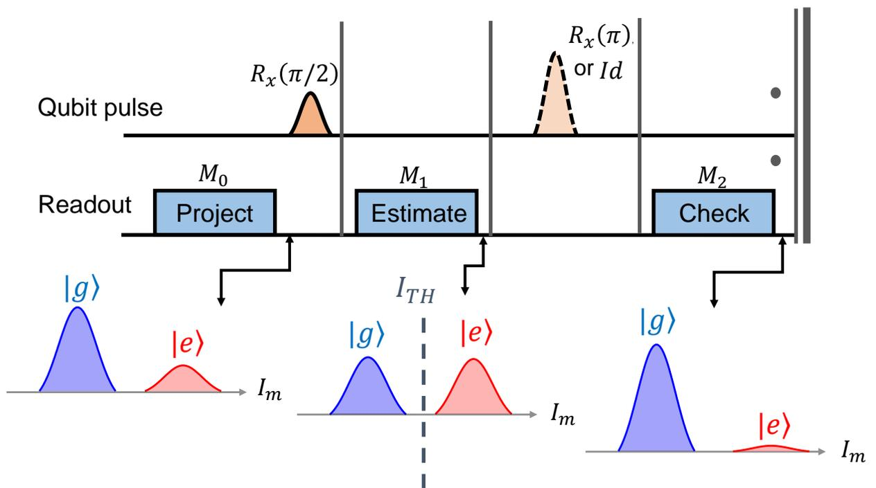
Figure 4.1: Pulse sequence of the baby Maxwell's demon.
