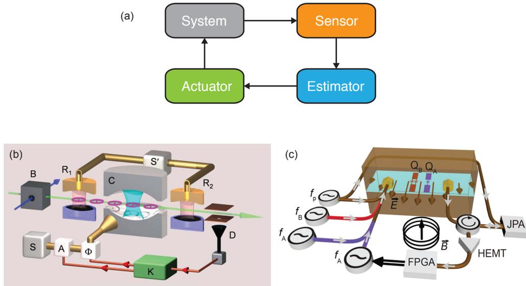
Figure 1.1: Overview of measurement-based feedback and examples. (a) The canonical flow of MB feedback loop. (b) Continuous MB feedback to stabilize a Fock state in a microwave cavity using Rydberg atoms, the first experimental demonstration real time quantum MB feedback[Sayrin et al., 2011]. (c) Deterministic entanglement generation of superconducting qubits by MB feedback[Riste et al., 2013].
