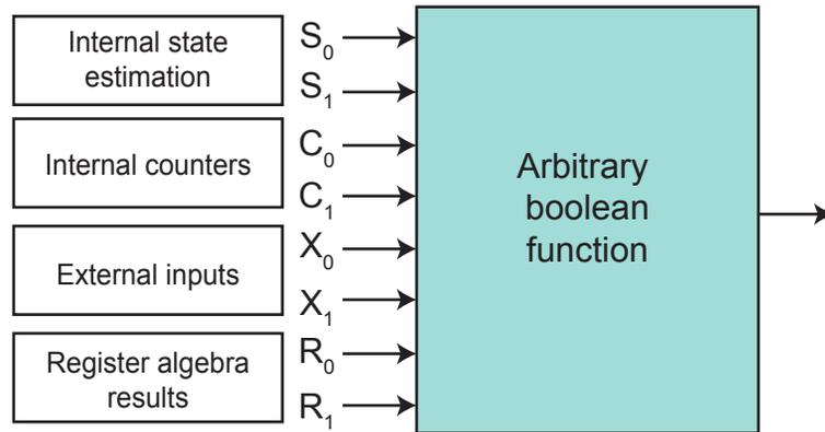
Figure 3.9: The *global state*, **internal result** is a boolean function of the states of eight 1-bit registers updated by the signals/processes shown in the boxes.
