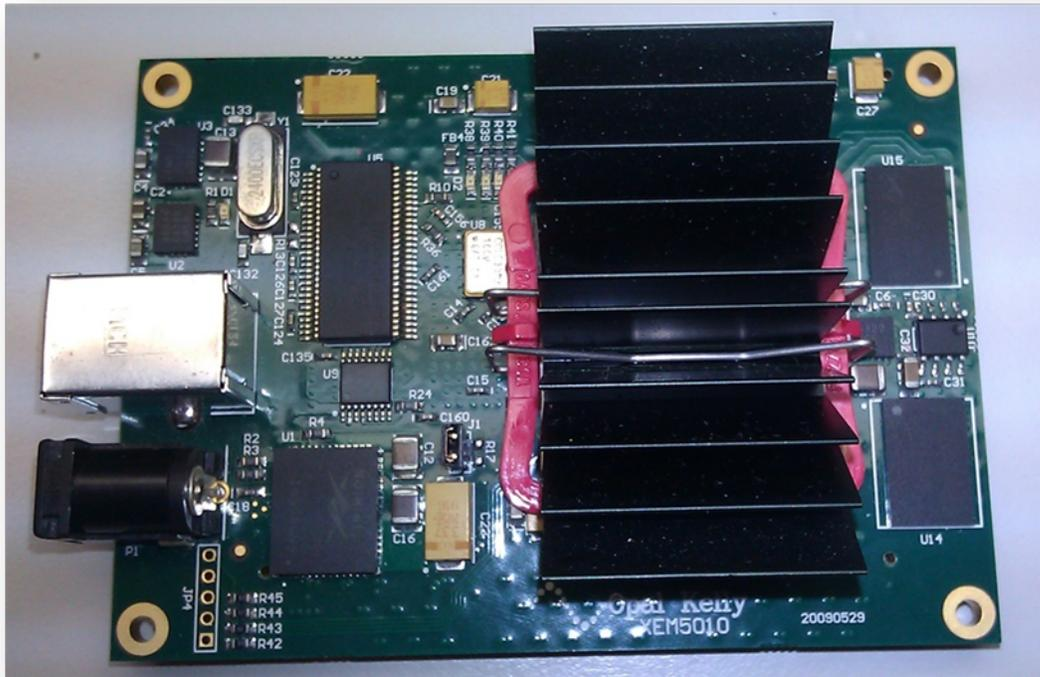
Figure 2.13: XEM5010 prototype board from Opal Kelly. The center piece of the first several generations of FPGA-enabled pulse generators developed. The large black meta looking piece is the heat sink underneath which sits the FPGA chip.
