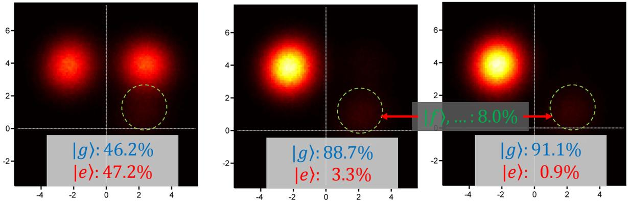
Figure 4.3: Measurement outcomes of repeating a stage of the baby Maxwell’s demon.
