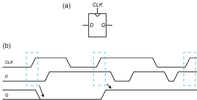
Figure 2.2: Register is the basic element of a synchronous FPGA logic circuit. (a) Schematic symbol of a register. (b) Timing diagram of a register. The input, *D*, is sampled and the output, *Q*, is updated on the rising edge of the clock exclusively. The output maintains its state at all other times.
