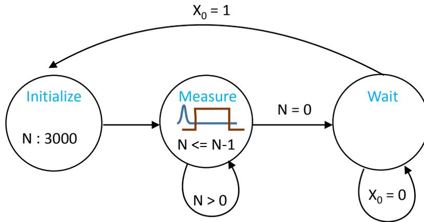
Figure 3.13: Constructing a FSM sequence for a spectroscopy experiment.
