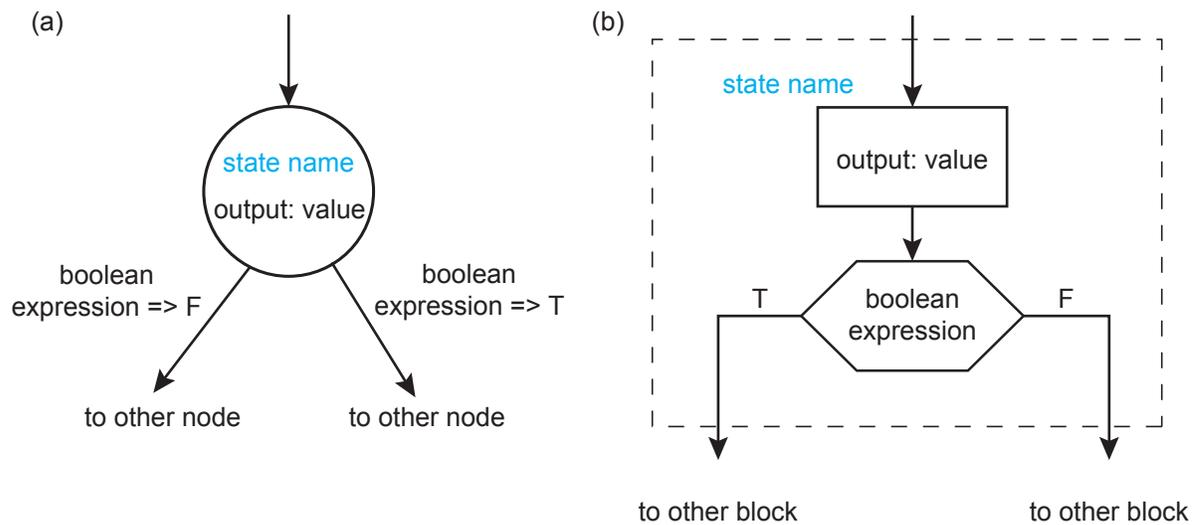
Figure 2.11: Two conventions of drawing a FSM state transition diagram. (a) a state diagram. (b) a algorithmic state machine (ASM) chart.
