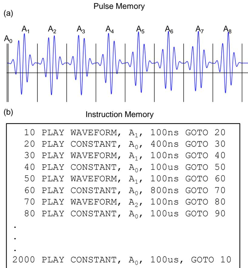
Figure 2.9: Construction of Pulse Memory and Instruction Memory. (a) Pulse memory is essentially a list of pulses. Each pulse is identified by the address of its first waveform point in the pulse memory, represented as  $A_n$  in the figure. (b) An pseudocode interpretation of an instruction memory, in the format specified in the previous figure.
