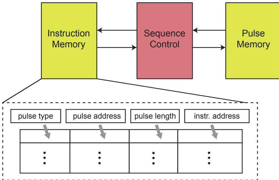
Figure 2.8: Architecture of a FPGA-based AWG. The three main components are the instruction memory, pulse memory and sequence control. Sequence control coordinates reading of both memories by specifying the locations to read from, i.e. memory addresses. The instruction memory is a table consisting of rows of instruction “words”, as shown inside the dashed box. Each word has four fields: three of them store values parametrizing a pulse and the fourth stores the location of the next instruction.
