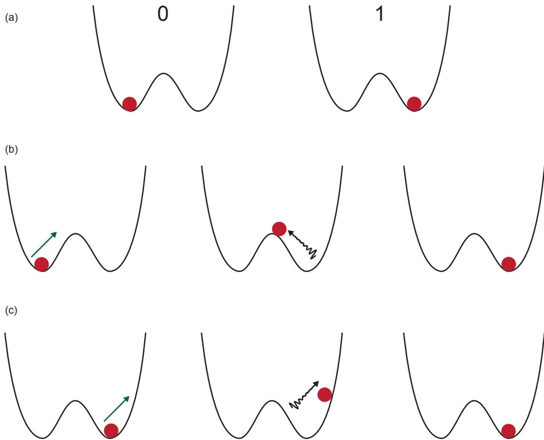
Figure 1.5: Resetting one bit of information. (a) Modeling a binary storage device as a double potential well. (b) Resetting a bit to "1" when it is initially "0". (c) Resetting a bit to "1" when it is initially "1".
