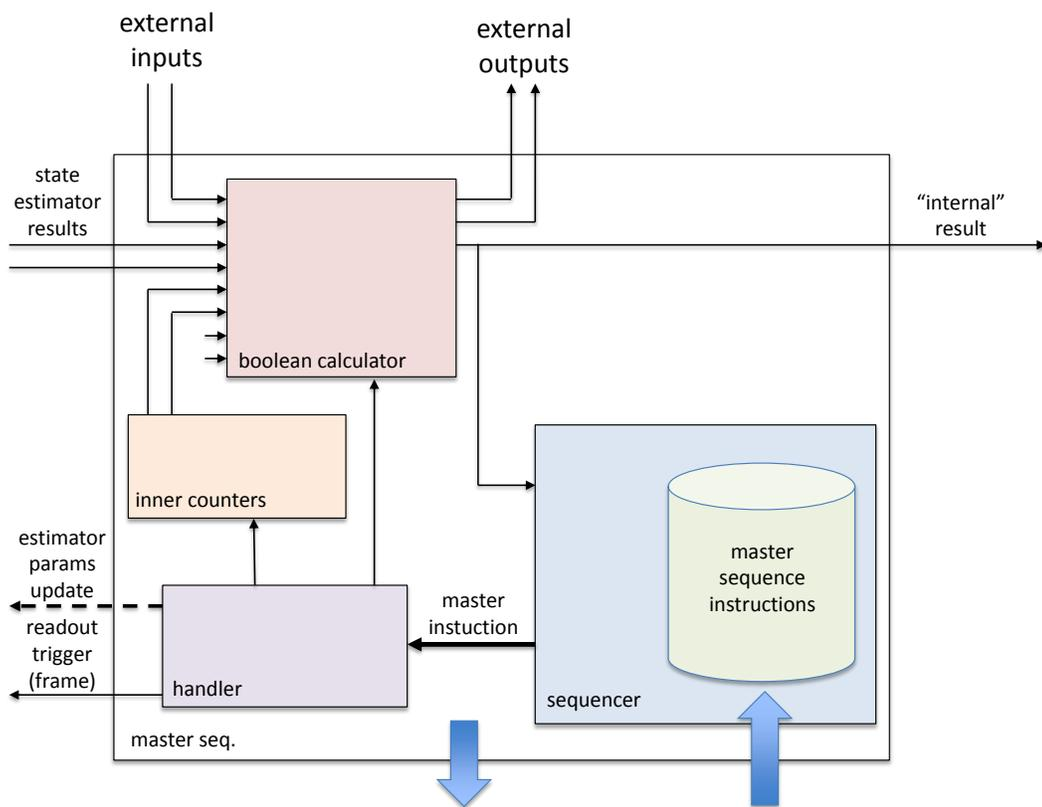
Figure 3.8: Architecture of the master sequencer.
