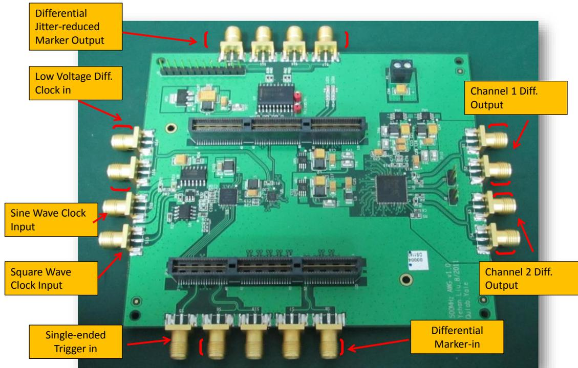
Figure 2.15: The 4th generation of FPGA-based AWG developed at Yale: 500MHz-AWG.
