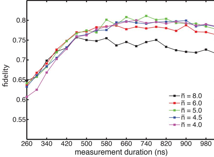
Figure 6.1: Experimental calibration of measurement strength and duration for MB. Fidelity to the state  $|\phi_+\rangle = \frac{1}{\sqrt{2}}(|ge\rangle + |eg\rangle)$  after preparing the qubits in a maximally superposed state followed by a quasi-parity measurement with post-selection. The fidelity is plotted as a function of measurement duration and shown for a set of measurement strengths. The optimal values chosen for the experiment are 660 ns and  $\bar{n} = 4.5$ .
