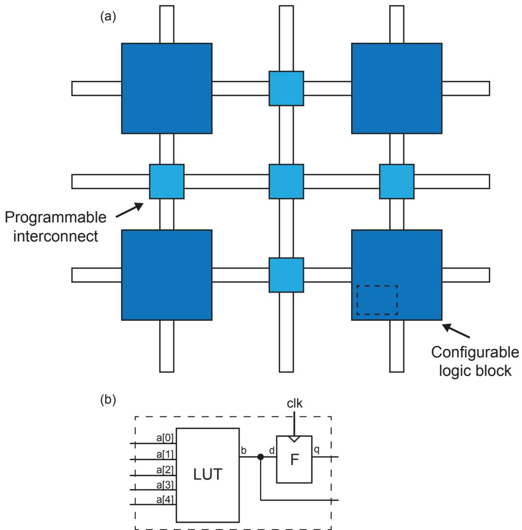
Figure 2.1: Schematic of a FPGA. (a) An FPGA is made up of a fabric of programmable logic blocks and switches between them (b) Inside each configurable logic block is several logic cells comprised of a look-up table and a flip-flop (register).
