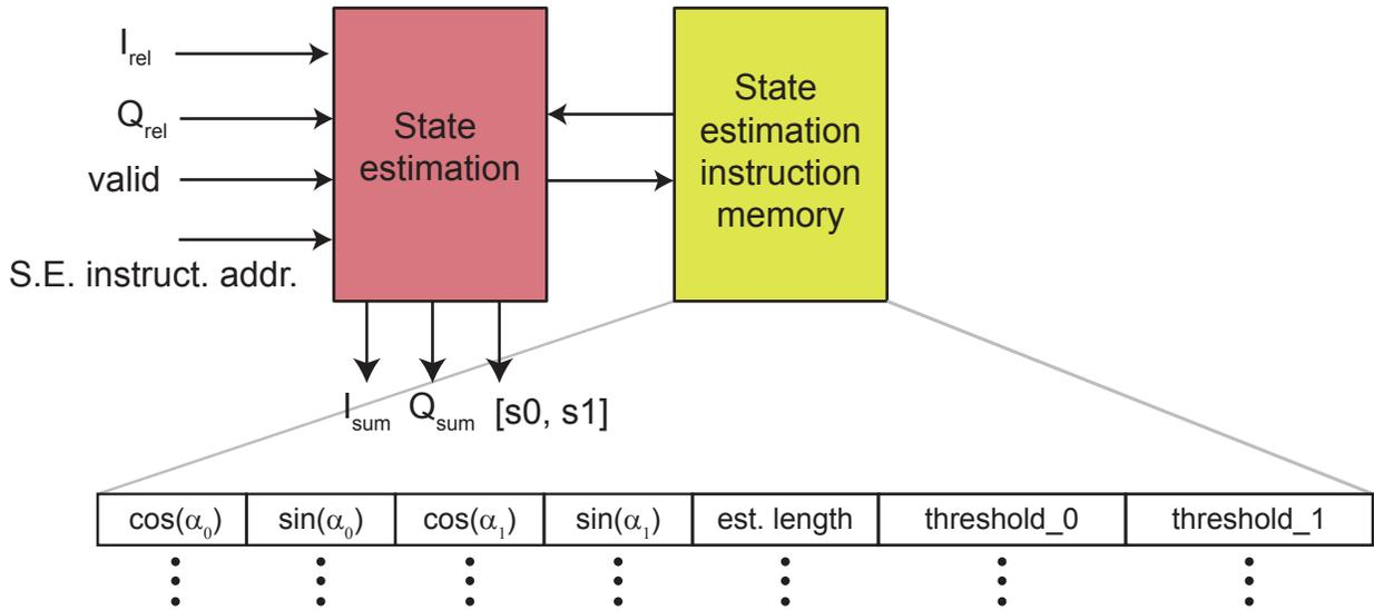
Figure 3.6: Architecture of the state estimator.
