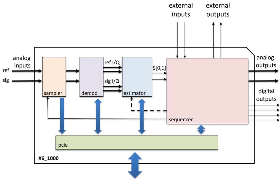
Figure 3.3: Architecture of the Yngwie logic for quantum feedback control.
