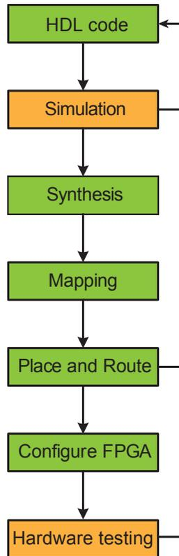
Figure 2.4: FPGA logic development flow. The flow chart describes the typical process of developing a FPGA logic circuit. Green blocks are actual design steps and yellow blocks are verification steps that are often necessary as well.
