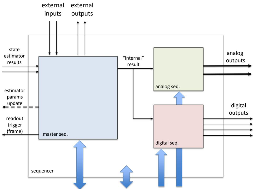
Figure 3.7: Top level architecture of the Yngwie Sequencer consisting of the master sequencer, analog sequencer and the digital sequencer.
