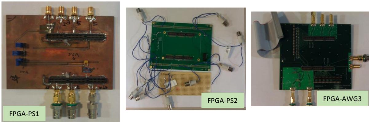
Figure 2.14: Early generations of FPGA-based pulse generators. The daughter- or expansion- boards were designed for the XEM5010 FPGA board.
