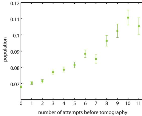
Figure 6.7: Experimental measurement of  $f$  state population plotted as a function of the boost attempts number in NFP for DD.
