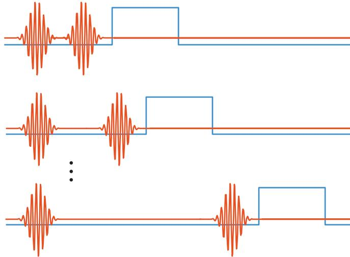
Figure 2.7: Pulse sequences for a T2 experiment, as required by a commercial AWG. The red waveforms are the qubit pulses and the blue waveforms are the digital marker pulses for modulating measurement drives. Every waveform point, including the parts with constant amplitudes, needs to be stored. This applies to both the analog and digital channels
