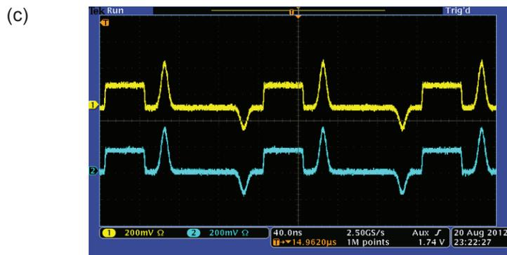
Figure 3.4: Clock domain crossing with FIFOs. (a) Yngwie logic is divided into three clock regions. (b) Both analog outputs jitter due to sample overflow/underflow when the middle region is not synchronized to a higher clock frequency and FIFOs for clock domain crossing are not used. (c) Jitter goes away when the proper changes introduced in the text are made.
