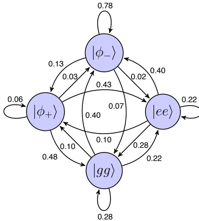
Figure 6.3: Markov model of a correction step in MB. Transition between any two nodes is possible and is represented as a directional edge. The 16 possible transitions make up the 16 matrix elements in the stochastic transition matrix,  $\mathcal{T}$ , corresponding to a correction step in MB. Numbers next to the edges represent the elements of  $\mathcal{T}$  calculated for the current experiment parameters by a master equation simulation.
