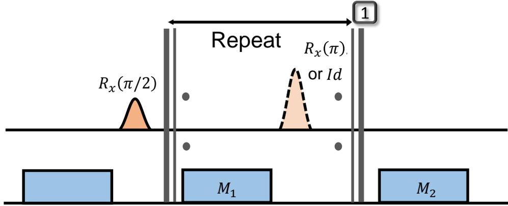
Figure 4.4: Repeating a stage of the baby Maxwell's demon
