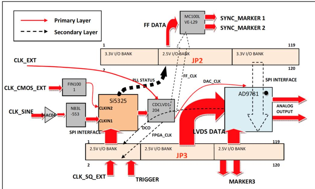
Figure 2.16: Signal routing of the 500MHz-AWG daughterboard
