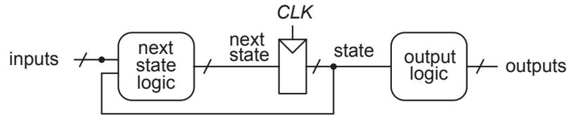
Figure 2.10: Logic circuit schematic of a FSM
