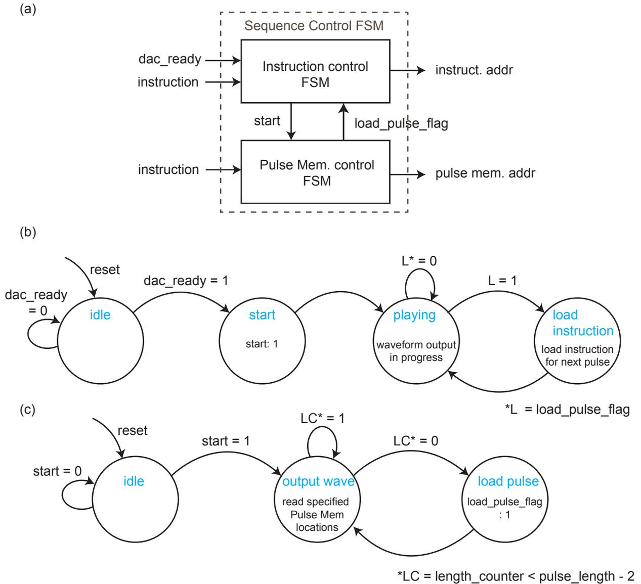
Figure 2.12: Implementation of the sequence control component of the FPGA-based AWG as a FSM. (a) A circuit schematic of the sequence control FSM implemented as two FSMs. (b) State diagram for the instruction memory control FSM which acts as the master. (c) State diagram for the pulse memory control FSM which is the slave.
