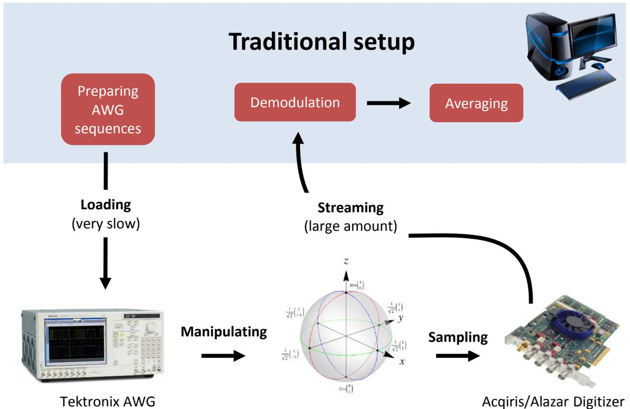
Figure 3.1: Traditional experimental setup for qubits control and measurement consists of three separate units. An AWG generates the control pulses to the quantum system. An analog-to-digital data acquisition card, such as an Alazar card, records the quantum system's responses. A computer is responsible for both generating the pulse sequences played on the AWG and for processing the record obtained by an Alazar.
