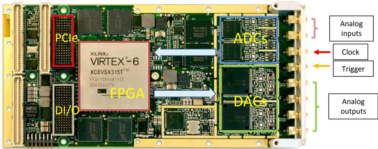
Figure 3.2: The X6-1000M FPGA board from Innovative Integration.
