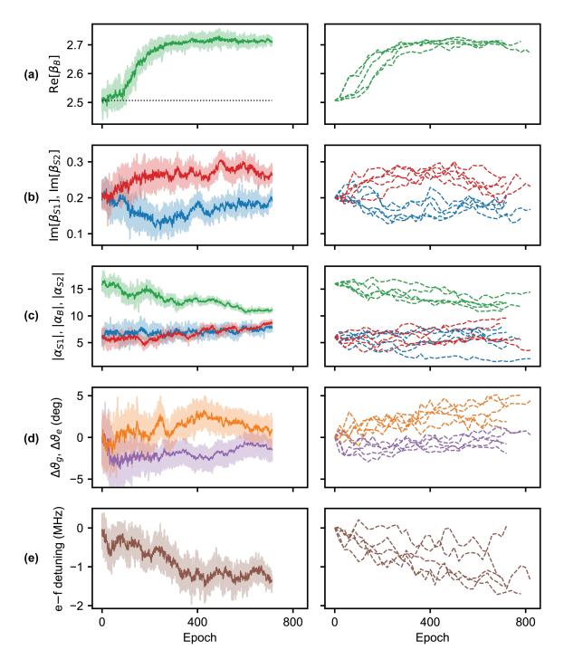
**Figure 6.4** | **Evolution of QEC circuit parameters during the training.** Top row: example from one particular training run. The shaded region bounds the minimal and maximal sampled parameter values. Solid lines indicate the mean. Bottom row: evolution of the mean parameter values in several independent training runs performed during a two-day period, showcasing the reproducibility of the training results.
