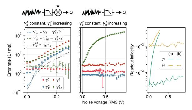
**Figure 6.13** | Noise verification experiments. (a) Component error rates as a function of the root mean square (RMS) voltage of the injected noise (at the generator plane). Here, noise is up-converted to the qubit frequency to increase  $\gamma_1^t$ . (b) Same as in (a), but with the baseband noise that increases  $\gamma_{\varphi}^t$ . (c) Readout infidelity of the transmon  $|g\rangle$  and  $|e\rangle$  states in these two noise injection settings.
