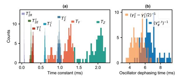
**Figure 4.5** | **Fluctuating error channels. (a)** Histogram of  $T_1$  and  $T_2$  times of the transmon and the oscillator, and logical lifetimes of error-corrected grid states. The histogram is derived from a week-long scan described in Chapter 6.10. (b) Oscillator pure dephasing time extracted from the measured oscillator parameters and predicted from the dispersive coupling model.
