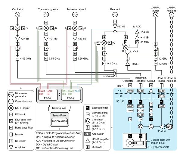
**Figure 3.2** | **Experimental setup.** For simplicity, the diagram omits DC ground connections of all active components, and attenuators placed at different locations at 300 K stage to ensure power levels within specs for amplifiers and switches.
