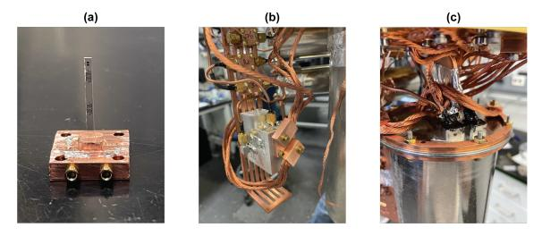
**Figure 3.1** | **Sample assembly. (a)** Clamped ancilla chip. **(b)** Thermalization. **(c)** Shielding.
