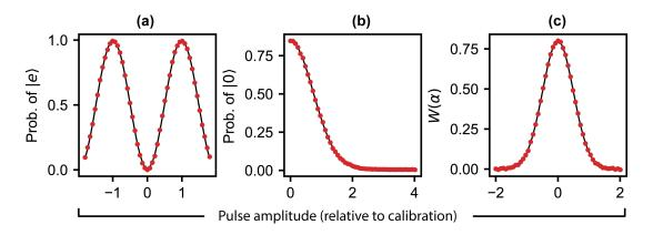
**Figure 4.1** | **Calibration of primitive pulses. (a)** Amplitude Rabi experiment to calibrate qubit rotations. **(b)** First-step calibration of displacement: probability of  $|0\rangle$  in a coherent state,  $P(0) = e^{-|\alpha|^2}$ . **(c)** Second-step calibration of displacement: Wigner function of vacuum,  $W(\alpha) = (2/\pi)e^{-2|\alpha|^2}$ .
