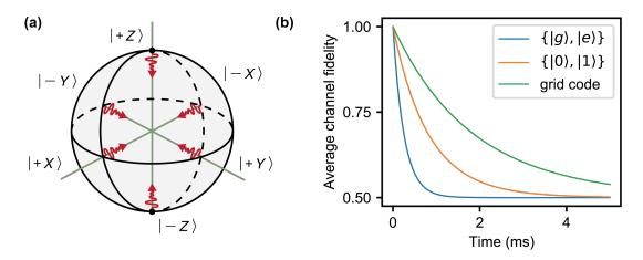
**Figure 6.15** | **Average channel fidelity. (a)** Illustration of channel action on the Pauli eigenstates. By linearity, the evolution of these six cardinal points is sufficient to predict the average effect across the whole Bloch sphere. **(b)** Expected time evolution of average channel fidelity for three different qubits, calculated using experimentally extracted lifetimes of Pauli eigenstates.
